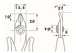
This type of shear cut, with slightly overlapping blades, due to the fact it does not exert mechanical stress, requires less force than that required by ordinary tools and results in reduced operator fatigue. A small measured cutting-edge misalignment is needed for the correct functioning of this tool.
